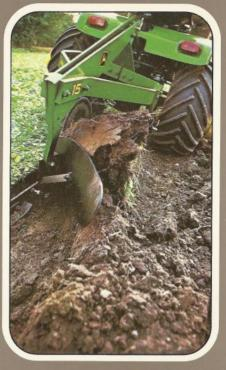
The 15 Plow is used on 300 Series and 400 Lawn and Garden Tractors. It works at depths of 4 to 8 inches with a 12-inch plow bottom. A 13-inch rolling coulter cuts sod or trash ahead of the plow.
