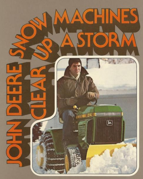
Front blades remove snow in winter and grade gravel drives in summer. Sizes range from 42 inches on the 100 and 200 Series to 54 inches on the 300 Series and 400. Box-beam construction makes these blades exceptionally durable.
