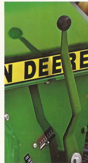
Manual lift (left) is standard. It provides excellent leverage for lifting attachments and can be locked in any of 7 positions. Electric lift (center) is optional. It has an exclusive position-responsive feature that moves the attachment in proportion to the movement of the lift lever. Hydraulic lift (right) provides power and durability for extra heavy work.
