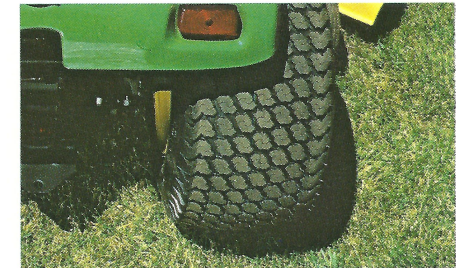
Wide turf tires provide a comfortable ride with less tire marking. Reversing rear wheels increases stability on hillsides.
