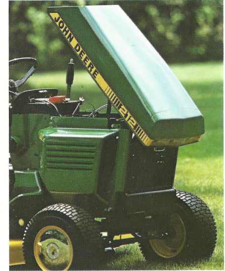
The rustproof hood tilts up for easy access to the engine compartment.
